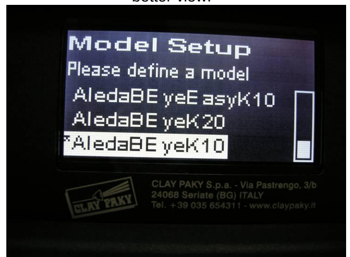
Insert the code "1234" and select "Setup Model", then select "A.leda B-EYE K10"
