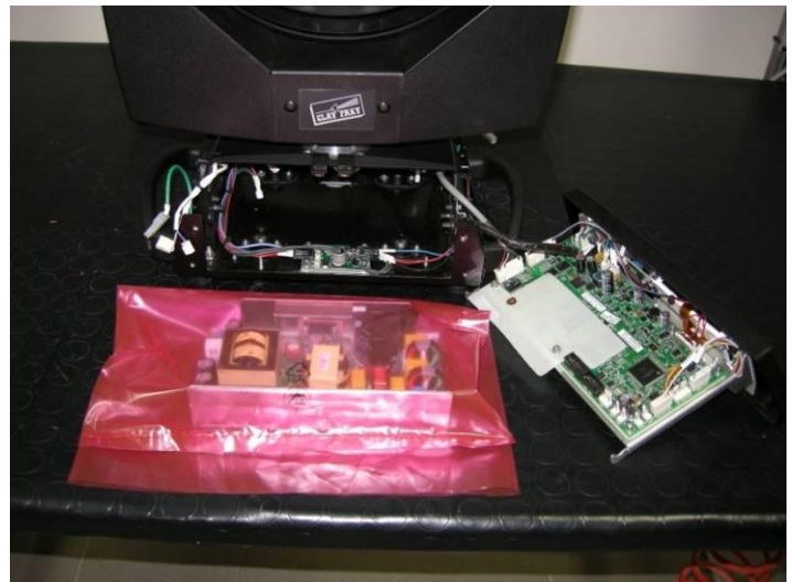
Rotate the main board assembly and slide out the CPU. Store the faulty part in an antistatic bag.
