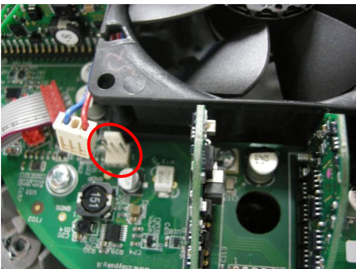
Move the fan on the new PCB, minding to orient it so that the connector faces its plug (circled)
