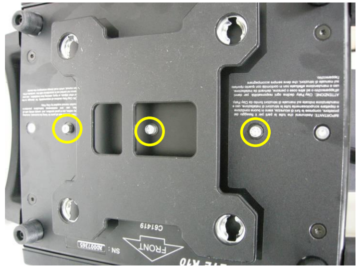
Flip the unit and remove the 3 circled screws.
