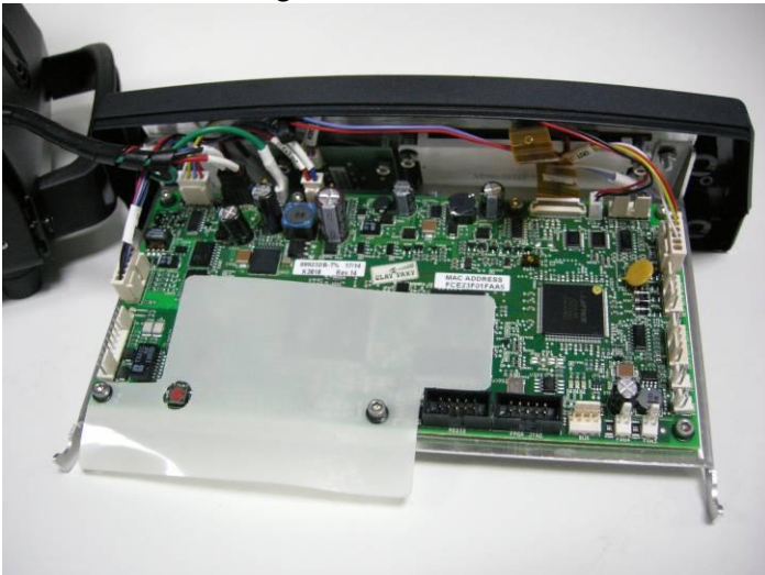
Plug back in all the other connections referring to the names on the wiring itself.
